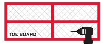
Screens or mesh must extend from the top rail to the walking/ working level and along the entire opening between rail supports.
